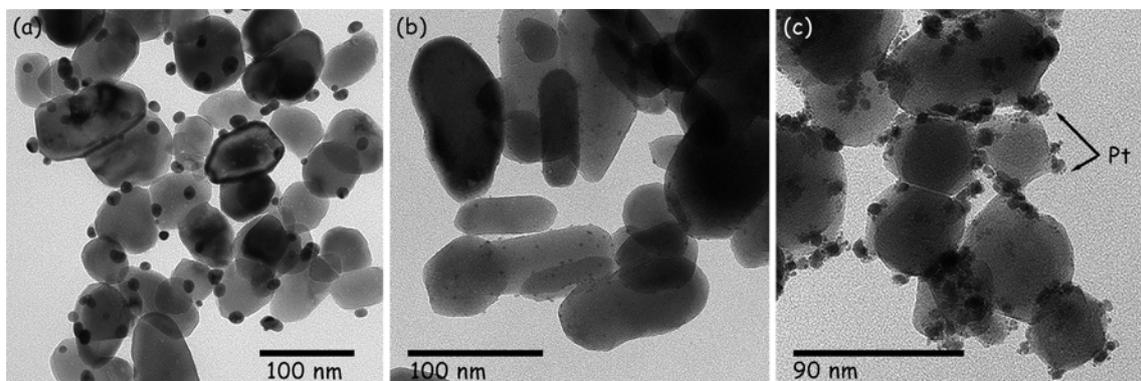
**Figure 1:** (a) TEM image of the as prepared Au-ZnO hybrid product. Au nanoparticles are ~10 nm in diameter. (b) TEM image of the as prepared Pt-ZnO hybrid product. (c) TEM image of the as prepared Pt-Au-ZnO hybrid product, where ~2 nm Pt nanoparticles are deposited on Au nanoparticles.
