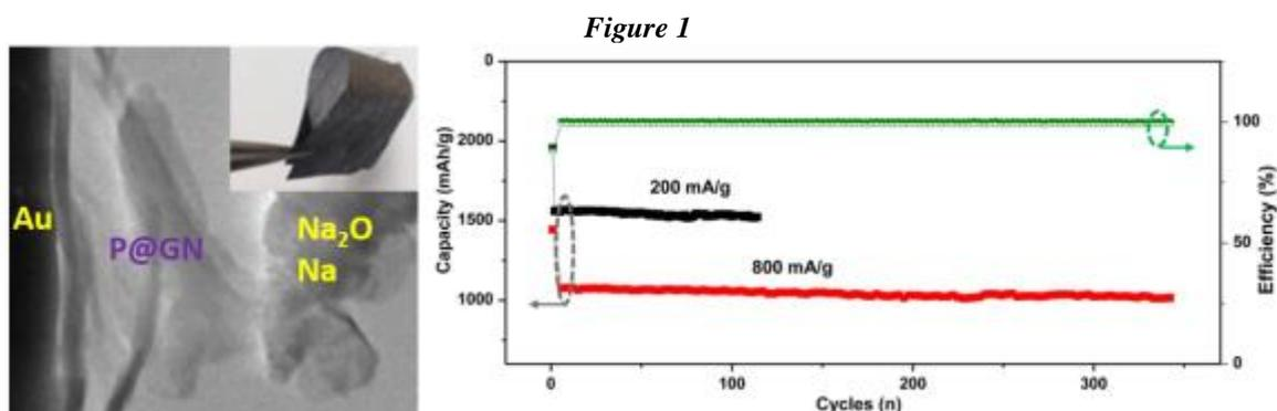
TEM image of the nano-SIB fabricated inside a microscope (the inset image shows the paper material for battery device fabrication), cyclic performance and Coulombic efficiency of P@GN at 200 mA/g and 800 mA/g.
